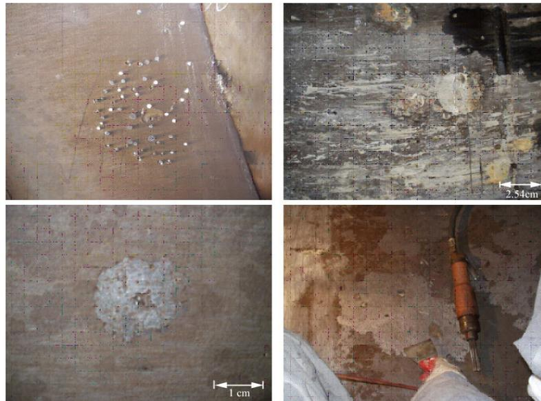
Fig. 1 Localized corrosion propagation after coating failures in seawater pipes
